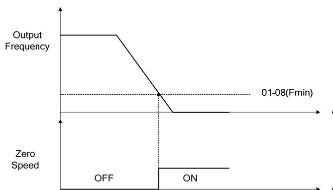
**Figure 4.4.23 Zero-speed operation**
