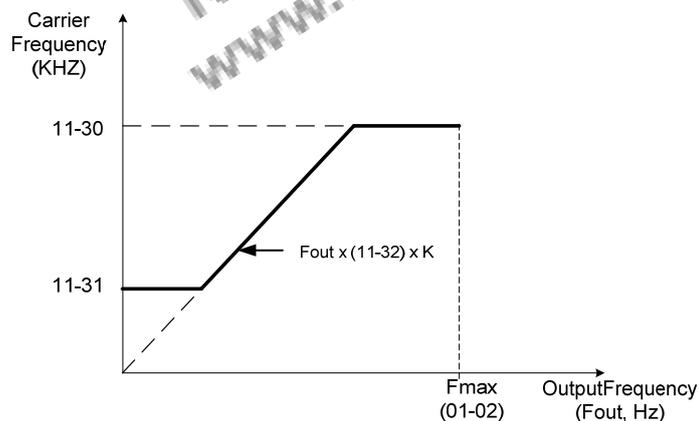
K is a coefficient; the value of K is based on the following based on the maximum carrier frequency:
