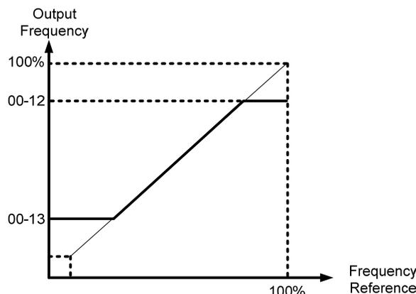
**Figure 4.4.5 Frequency reference upper and lower limits**
