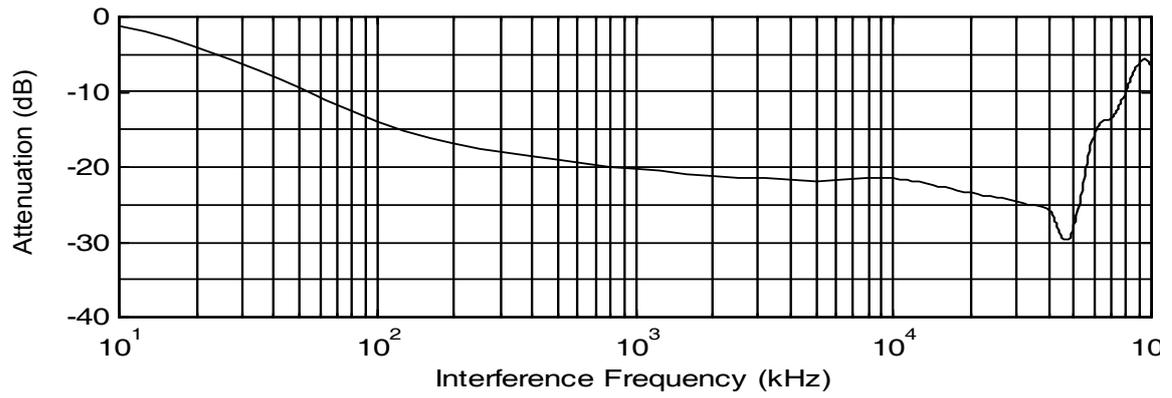
Figure 11.3.1 Frequency attenuation characteristics (10 windings case)
