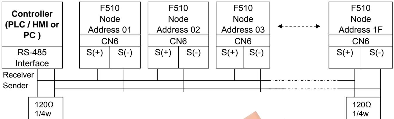
\*\*The distance of communication line with above 200m should have terminal resistors, which ought to be placed at both ends, so as to eliminate reflection phenomenon. \*\*
