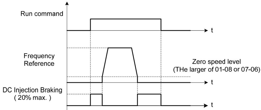
Figure 4.4.84 Zero-speed braking operation
