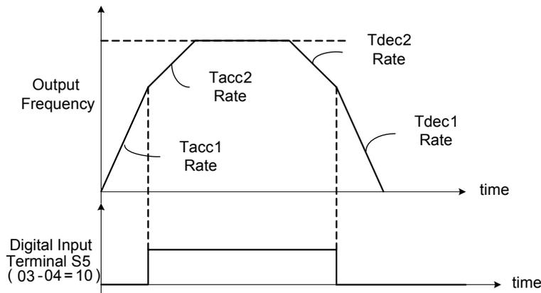
**Figure 4.4.6: Terminal S5 switch between Tacc1/Tacc2 and Tdec1/Tdec2**
