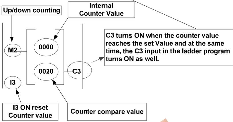
C3 turns ON when the counter value reaches the set Value and at the same time, the C3 input in the ladder program turns ON as well.
