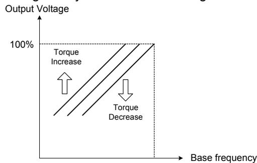
**Figure 4.4.11 Torque compensation gain to increase/decrease output torque**
