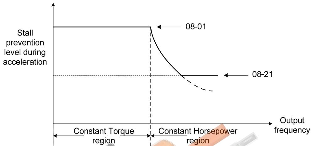
**Figure 4.4.58 Stall prevention level and limit in acceleration**
