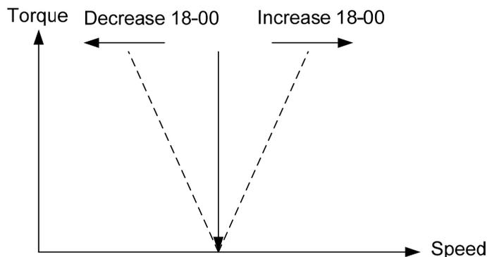
**Figure 4.4.92 18-00 Effect on the torque and speed**
