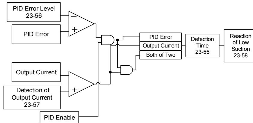
**Figure 4.4.115 Diagram for the process of low suction**
