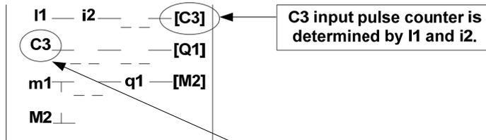
C3 input pulse counter is determined by I1 and I2.
