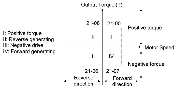
**Figure 4.4.101 Torque limit setting**
