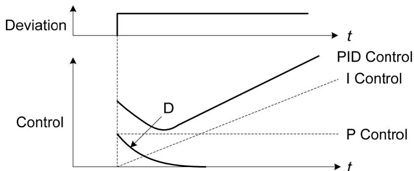
Figure 4.4.68 PID Control
