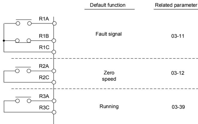
Figure 4.4.22 Multi-function digital output and related parameters
