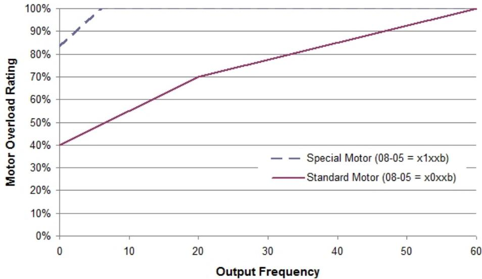
Figure 4.4.62 Motor overload rating at different output frequencies
